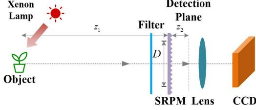
FIG. 2. Experimental setup of lensless Wiener-Khinchin tele-scope.
