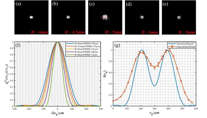
FIG. 4. Resolution at different apertures of the spatial random phase modulator. Reconstructed images with different apertures: (a)  $D = 4 \text{ mm}$ , (b)  $D = 4.5 \text{ mm}$ , (c)  $D = 5 \text{ mm}$ , (d)  $D = 6 \text{ mm}$ , (e)  $D = 8 \text{ mm}$ . (f) The theoretical resolutions. (g) A comparison between theoretical and experimental resolutions at  $D = 5 \text{ mm}$ , and the red line is a cross-section denoted by the dash line in Fig. 4(c).
