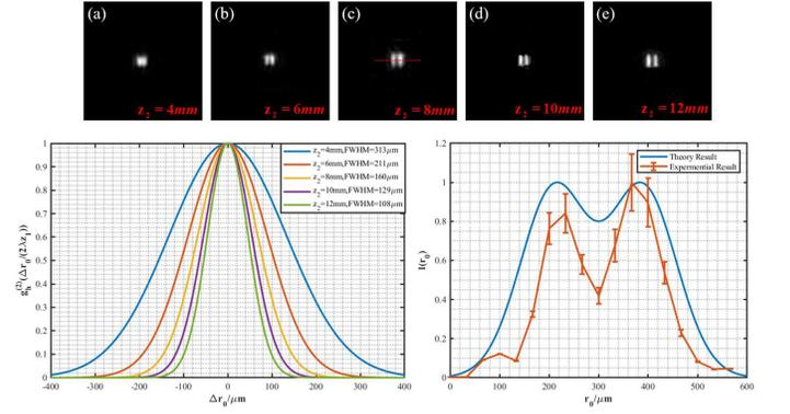
FIG. 5. Resolution at different  $z_2$ . Reconstructed images with different  $z_2$ : (a)  $z_2 = 4 \text{ mm}$ , (b)  $z_2 = 6 \text{ mm}$ , (c)  $z_2 = 8 \text{ mm}$ , (d)  $z_2 = 10 \text{ mm}$ , (e)  $z_2 = 12 \text{ mm}$ . (f) The theoretical resolutions. (g) A comparison between theoretical and experimental resolutions at  $z_2 = 8 \text{ mm}$ , and the red line is a cross-section denoted by the dash line in Fig. 5(c).
