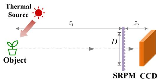
FIG. 1. Schematic of a lensless Wiener-Khinchin telescope.  $D$  is the diameter of the SRPM.  $z_1$  and  $z_2$  are distances from the object and detection planes to the SRPM, respectively.
