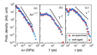
FIG. 3. Statistical distributions of the (a) stress drop, (b) duration, and (c) waiting time of plastic deformation (avalanche) events. The distributions obtained from the as-quenched and well-aged models are represented by red squares and blue circles, respectively.
