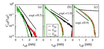
FIG. 5. Spatial correlation functions of the nonaffine squared displacement at  $\dot{\gamma}t$  values of (a) 0.0765, (b) 0.0960, and (c) 0.0988, where the functions at  $\dot{\gamma}t=0.0765$  and 0.0960 are obtained from the as-quenched model and that at  $\dot{\gamma}t=0.0988$  is obtained from the well-aged model. The correlation functions along the xy,yz, and zx planes are depicted by the red, blue, and green lines, respectively.
