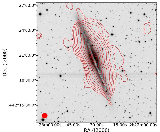
**Fig. 4.** LOFAR map of NGC 891 at a resolution of  $40.0'' \times 35.7''$  shown by the filled ellipse in the bottom left, overlaid onto an optical image from the Digitized Sky Survey. Contours are at 3, 5, 8, 12, 18, 32, 44, 88, 164,  $200 \times \sigma$  where  $\sigma = 1.1$  mJy/beam is the rms noise level.
