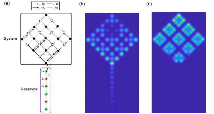
**Supplementary Figure 6.** (a) Schematic showing the topological “system” and the non-Hermitian “reservoir”. (b,c) Two zero modes that couples and does not couple to the reservoir, respectively.
