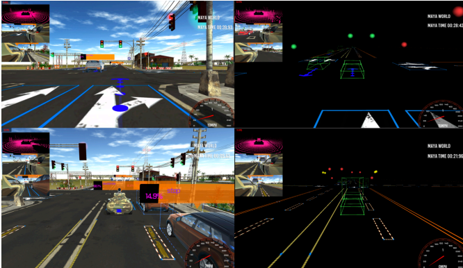
Figure 2: Scene of urban driving is shown both in regular rendering and “skeleton” mode with traffic lights, HD map information provided.
