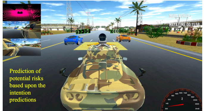
Figure 6: Demonstration of the prediction of potential risks is shown where a conflict of interests on a spot between two vehicles are predicted based upon the intention prediction results. The risky zone or spot is marked by the yellow warning box on the road surface.
