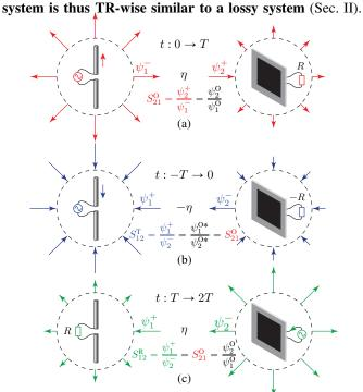
Fig. 2. TRA and apparent (restricted) nonreciprocity of an open system composed of a dipole antenna and a patch antenna in free space.
