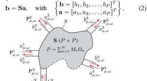
Fig. 3. Arbitrary P-port network and extended scattering matrix, S.
