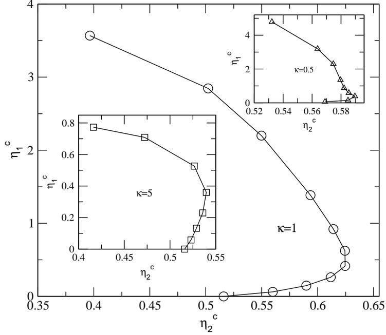
FIG. 5: The respective packing fractions of the two species at the ENE transition points of MCT,  $\{\eta_1^c, \eta_2^c\}$  for a hard sphere mixture of size ratio  $\alpha = 10$  and mass ratio  $\kappa = 1$ (main),  $.5$  (upper inset), and  $5$  (lower inset). Reentry of the critical behavior with respect to  $\eta_2^c$  is seen here since at a fixed  $\eta_2^c$ , two possible values of  $\eta_1^c$  occur.
