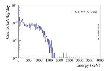
**Figure 2.** Summed background spectrum from DS3 and DS4 after all cuts (enriched Ge detectors only). One count remains in the 400-keV region of interest centered at the 2039-keV  $0\nu\beta\beta$  Q value.
