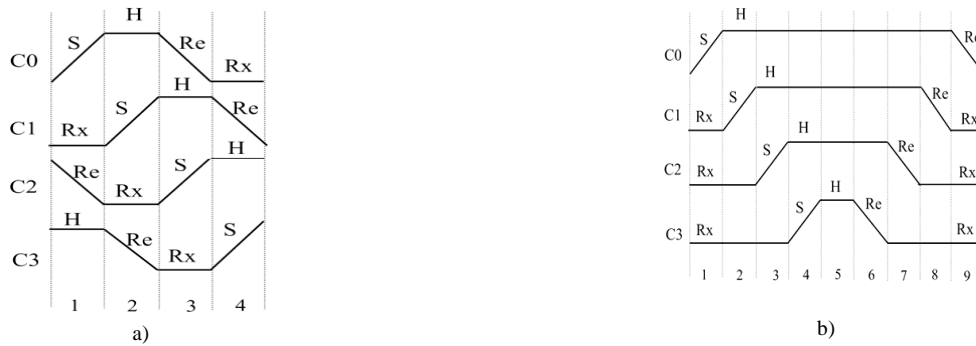
Fig. 4. a) Landauer clocking waveform. b) Bennett clocking waveform. S: switch phase, H: hold phase, Re: release phase, Rx: relax phase.
