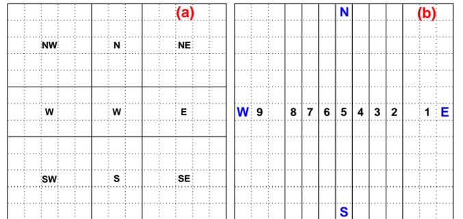
FIG. 1: (a) 9 directions (FOV = 2.3 sr.) used earlier [1]. (b) a new combination of 169 directions labeled 1 through 9 with an angular segmentation of  $10.6^\circ$  used here.
