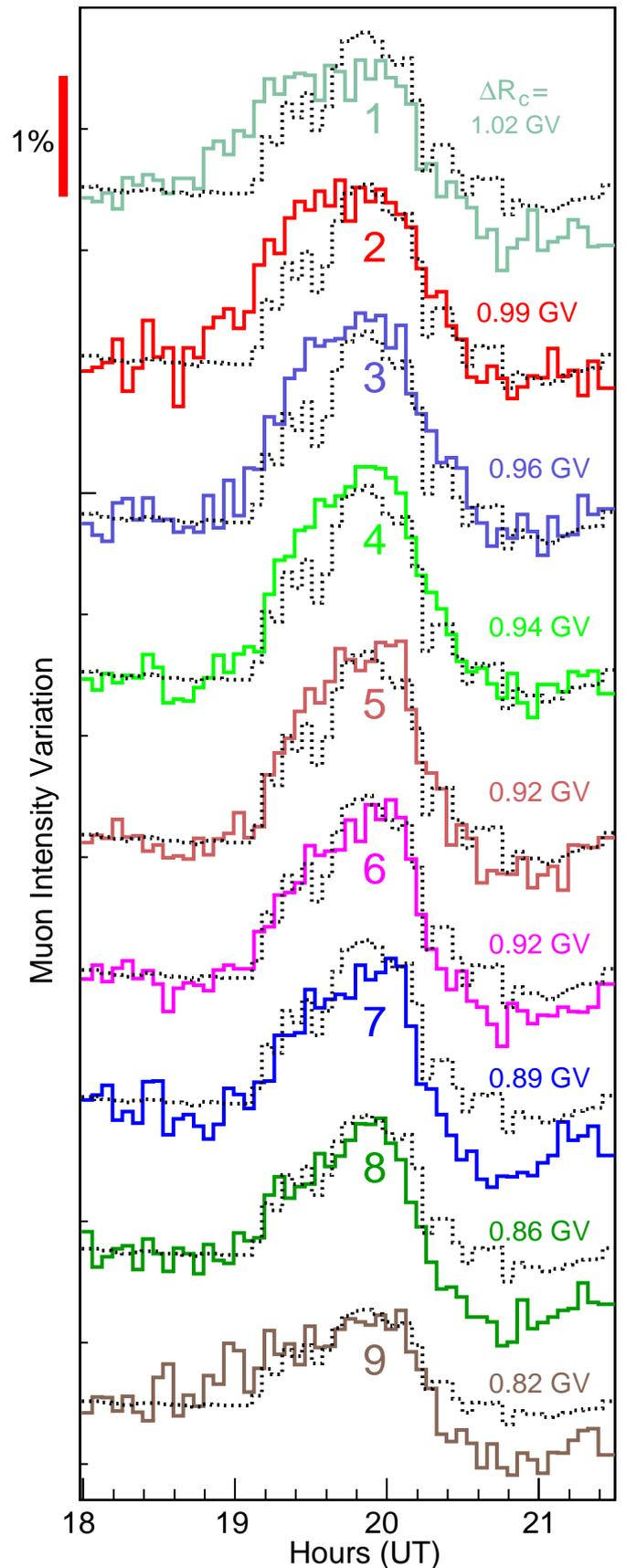
FIG. 4: Muon intensity variation observed by GRAPES-3 on 22 June 2015 in nine directions labeled ‘1’ in East through to ‘9’ in West. Monte Carlo simulation for each direction is shown by dotted lines.
