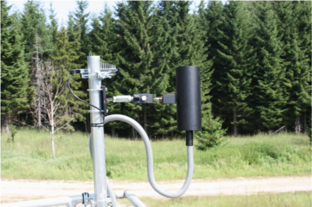
Figure 1. Example for the setup of the Upper Austrian NSB measurement net at Zöbelboden (ZOE). The black cylinder is the waterproof SQM housing.
