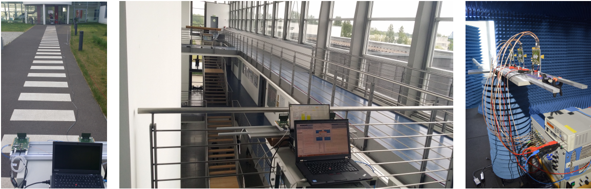
Fig. 1. Three example measurement scenarios. Left: outdoor 2 \times 2 scenario, FE1, link distance between 10 m and 60 m. Center: indoor short-range backhaul 2 \times 2 scenario, FE1, distance of 15 m. Right: anechoic chamber 3 \times 3 scenario, FE2, distance of 5 m.
