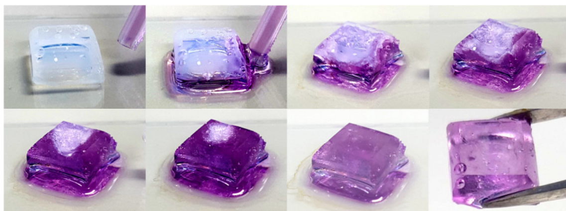
Figure 2. Photographs showing the imbibition of a mesoporous silica stamp with a solution of \text{C}_{60} in toluene (pink). The mesoporous silica stamp with edge lengths of \sim 5 mm is located on a glass slide in such a way that the contact surface of the mesoporous silica stamp topographically patterned with the contact elements points upwards. Prior to imbibition, the empty mesoporous silica stamp is opaque and colourless. The \text{C}_{60} /toluene solution dropped onto the glass slide close to the mesoporous silica stamp invades the latter. The portions of the mesoporous silica stamp filled with \text{C}_{60} /toluene solution are transparent-pink.
