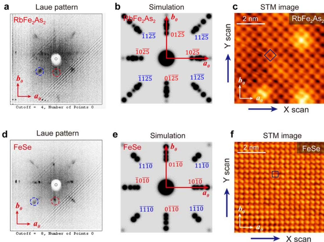
**Figure S5** | Determine the surface lattice orientation of  $\text{RbFe}_2\text{As}_2$  by Laue diffraction and STM imaging. (a) Laue diffraction pattern of  $\text{RbFe}_2\text{As}_2$  single crystal. (b) Simulated Laue pattern using SingleCrystal™ software for  $\text{RbFe}_2\text{As}_2$  with  $a_0$ ,  $b_0$  along X and Y directions. The Miller indices (hkl) of the planes corresponding to the diffraction points near center are marked, which are belong to  $\{01X\}$  (red) and
