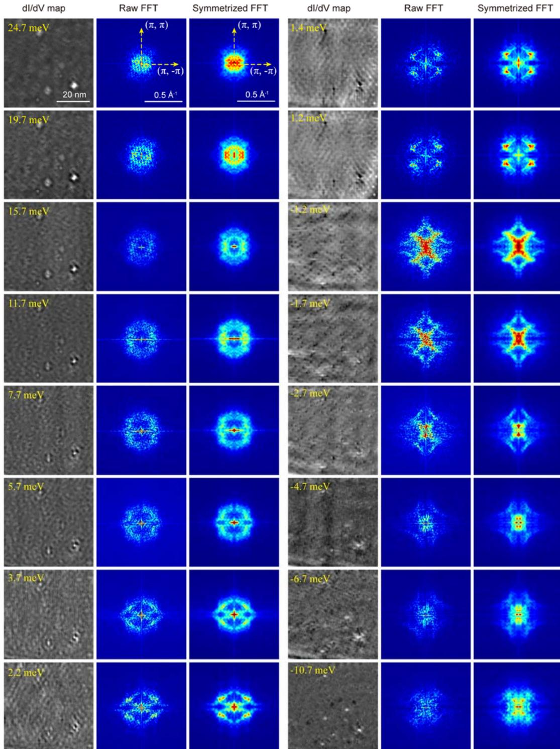
**Figure S7 | A full set of  $dI/dV$  maps taken on type A surface and their FFTs.** The topography of the mapping area is shown in Fig. 1b. Each  $dI/dV$  maps are taken at a  $V_b$  equal to the mapping energy (labeled on the map) and  $I = 100\text{pA}$ ; the lock-in modulation ( $\Delta V$ ) for each map has an amplitude of 5%  $V_b$ . Details about the FFT symmetrization is described above. Every  $dI/dV$  map has  $256 \times 256$  pixels.
