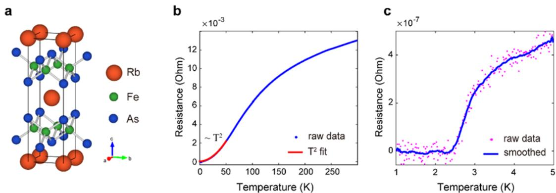
**Figure S1** | (a) Bulk crystal structure of  $\text{RbFe}_2\text{As}_2$ . (b) Temperature dependence of the resistance ( $0 \sim 300\text{K}$ ), the red curve below 50 K is a fit to  $T^2$ . (c) Temperature dependence of the resistance across the superconducting transition at  $T_c \sim 2.5\text{K}$ .
