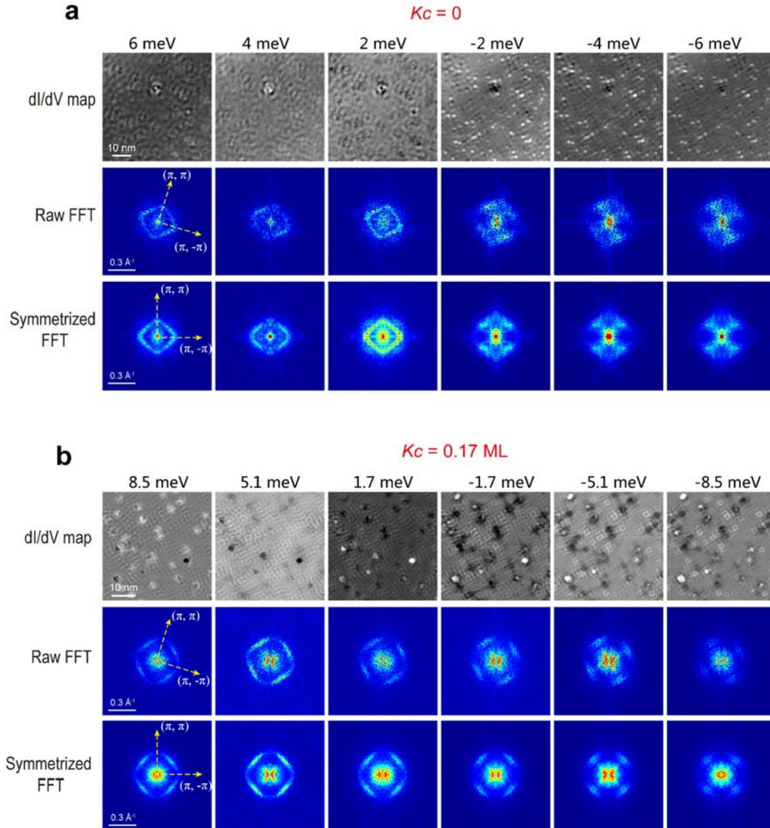
**Figure S9 |** (a) Additional dI/dV maps, raw FFTs and symmetrized FFTs taken on RbFe<sub>2</sub>As<sub>2</sub> with K<sub>c</sub> = 0 at T = 4.5K. All dI/dV maps are taken at the setpoint of V<sub>b</sub> = 10mV, I = 200pA, ΔV = 1mV. (b) Additional dI/dV maps, raw FFTs and symmetrized FFTs taken on RbFe<sub>2</sub>As<sub>2</sub> with K<sub>c</sub> = 0.17 ML at T = 4.5K. All dI/dV maps are taken at the setpoint of V<sub>b</sub> = 10mV, I = 200pA, ΔV = 1mV. Each map has 250 × 250 pixels.
