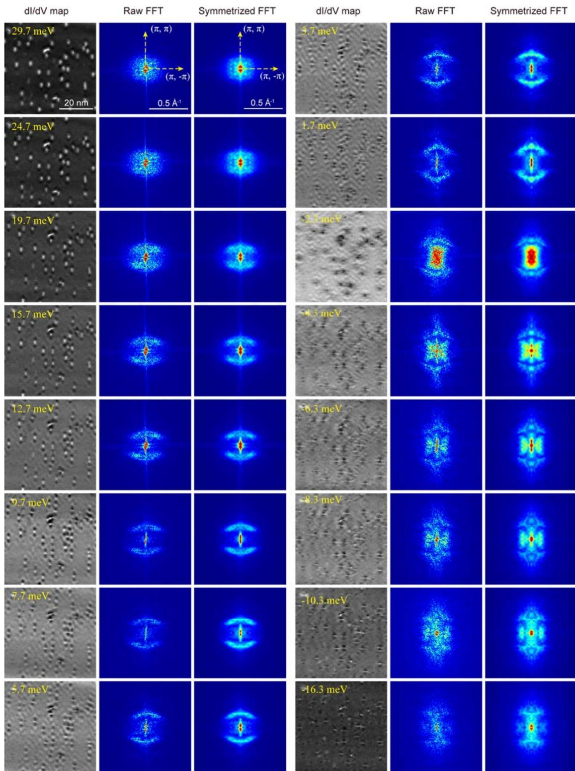
**Figure S8 | A full set of  $dl/dV$  maps taken on type B surface and their FFTs.** The topography of the mapping area is shown in Fig. 1c. Each  $dl/dV$  maps are taken at a  $V_b$  equal to the mapping energy (labeled on the map) and  $I = 100\text{pA}$ ; the lock-in modulation ( $\Delta V$ ) for each map has an amplitude of 5%  $V_b$ . Every map has  $256 \times 256$  pixels.
