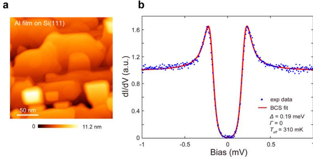
**Figure S2** | (a) Topographic image of an Al/Si(111) film of thickness  $\sim 20$ ML. (b) The superconducting gap of the Al/Si(111) film taken at  $T = 20$  mK ( $V_b = 1$  mV,  $I = 100$  pA,  $\Delta V = 30$   $\mu$ V). Red curve is the BCS fit with  $\Delta = 0.19$  meV,  $T_{eff} = 310$  mK and  $\Gamma = 0$ .
