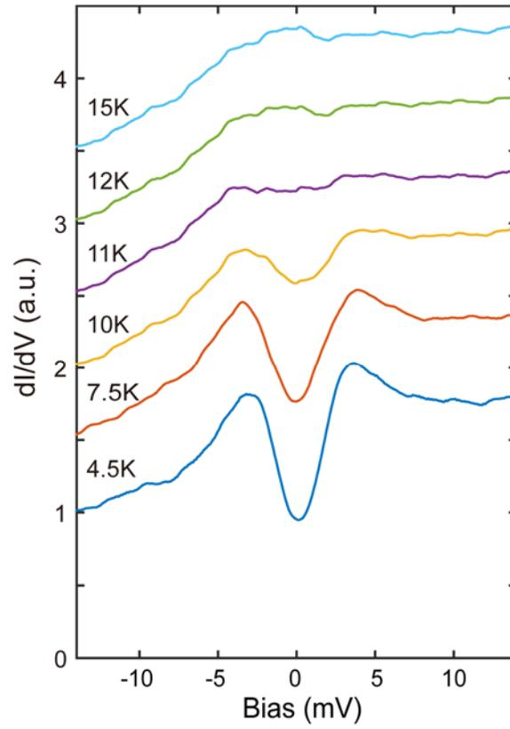
**Figure S10** | Temperature dependence of the low energy tunneling gap observed at  $K_c = 0.17$  ML ( $V_b = 15$  mV,  $I = 300$  pA,  $\Delta V = 1$  mV for all the spectra). The gap closed at about 12K.
