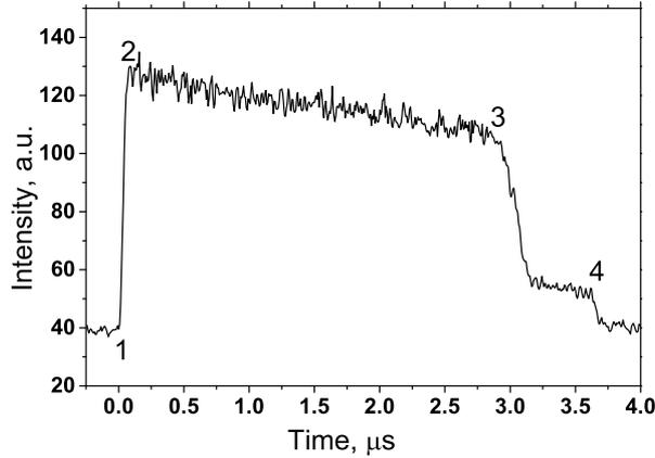
**Figure 3.** Time dependence of the light emission out of a shock-compressed xenon plasma: 1—shock wave exit on the free surface of a charge; 2—end of increase of optical thickness of shock compressed plasma; 3—beginning of reflection of shock wave front from the flange; 4—back side of detonation products arrived at the flange.
