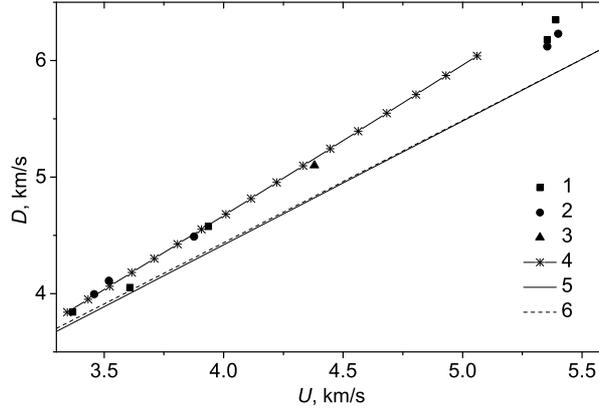
**Figure 5.** Hugoniot of xenon in  $D$ - $U$  coordinates: 1—experiment at initial pressure 5 bar [22]; 2—experiment at initial pressure 10 bar [22]; 3—experiment at initial pressure 10 bar [4]; 4—approximation of experimental data in present work at initial pressure 7 bar; 5—Debye approximation in a grand canonical ensemble of shock-compressed xenon at initial pressure 5 bar [22]; 6—Debye approximation in a grand canonical ensemble of shock-compressed xenon at initial pressure 10 bar [22].
