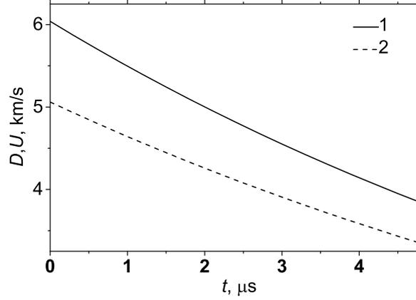
**Figure 4.** Time dependent approximation of  $D(t)$  and  $U(t)$ : 1—velocity of shock wave front; 2—velocity of shock compressed plasma.
