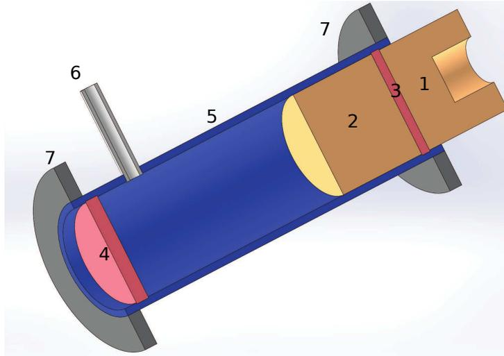
**Figure 1.** Cross view of shock tube of non-ideal plasma for proton radiography: 1—intermediate charge with a hole for a detonator; 2—active charge; 3—flange for high explosive; 4—transparent flange; 5—shock tube channel; 6—gas inlet; 7— fastening rings.
