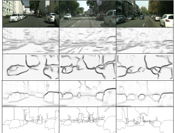
Figure 10: Edge detection results on Cityscapes dataset. From top to bottom: input image, unsupervised edge by Li et al. [36], HED-N, our results, edge ground truth. All detection visualization results are before the process of non-maximum suppression).
