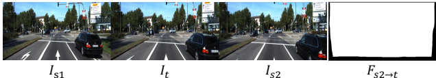
Figure 4: Some part of the scene flies out as camera moves forward from I_t to I_{s2} . A fly-out mask is calculated from camera motion to filter out such regions.
