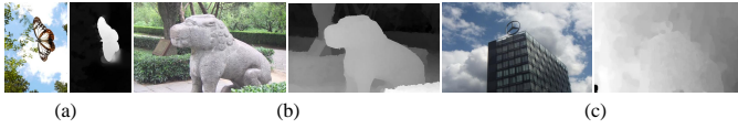
Fig. 5. Different quality depth maps. (a) Good depth map, \lambda_d = 0.8014 . (b) Common depth map, \lambda_d = 0.3890 . (c) Poor depth map, \lambda_d = 0.0422 .
