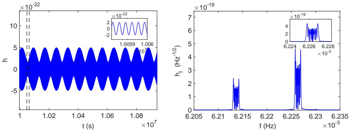
**Figure 3.** Left panel: Clip of the one-year noiseless time series of the strain output of a Michelson interferometer for GWs from the reference source. The inset zooms in of the data segment within the double dash lines. Right panel: ASD of the time series. The inset zooms in the right horn.
