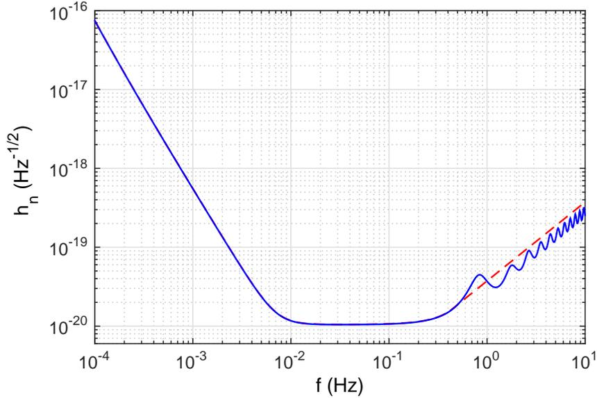
**Figure 2.** Sensitivity curve of TianQin. The blue solid line is the numerical evaluation of Eq. 16 over the interested frequency range. The red dash line is obtained from an analytic approximation. The two lines overlap for  $f < f_* \approx 0.28$  Hz.
