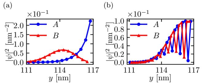
FIG. 3. (Color online) Square modulus of the electron wave function for  $E_F = 4\Delta_0$  along the  $y$ -direction for the ZC (a) and AC (b), close to the top edge of graphene [panel (b) is a vertical cut of Fig. 4(a) taken at  $x \simeq 14$  nm]. All other parameters are the same as for Fig. 2.
