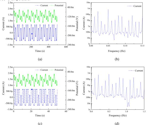
and 0.01 Hz and with amplitude of 10 mV and system responses in time domain and frequency domain at 90°C temperature.
