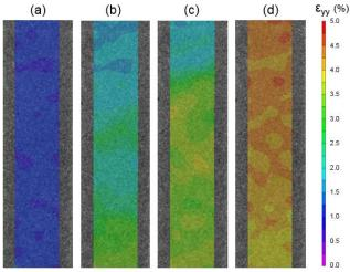
Figure 3. Strain distribution in loading direction ( $\epsilon_{yy}$ ) corresponding to (a) 1%, (b) 2%, (c) 3%, and (d) 4% applied strain.
