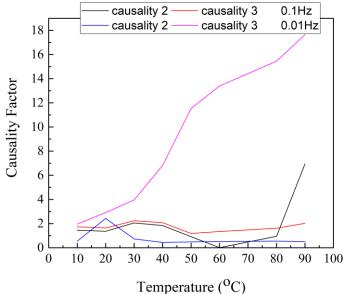
Figure 6- Influence of the temperature on the causality factors are calculated for base frequencies 0.1 and 0.01 Hz.
