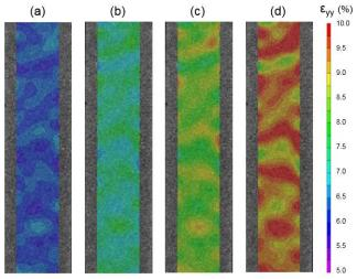
Figure 4. Strain distribution in loading direction ( $\epsilon_{yy}$ ) corresponding to (a) 6%, (b) 7%, (c) 8%, and (d) 9% applied strain.
