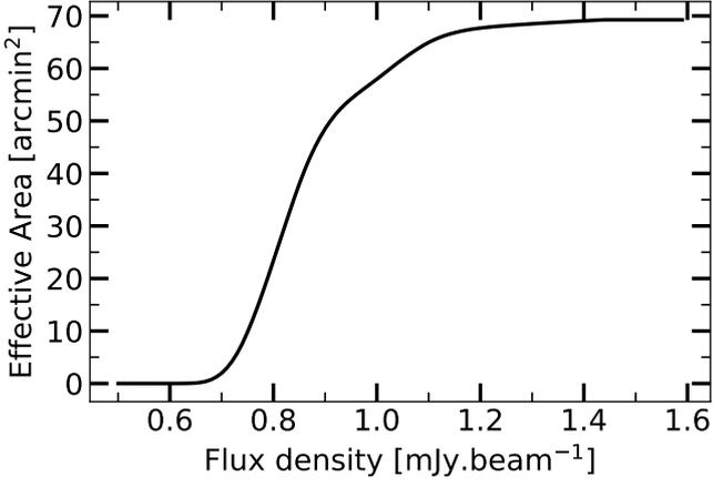
**Fig. 14.** Effective area as a function of flux density, where a source with a given flux can be detected with an SNR  $> 4.8\sigma$ . Ninety percent of the survey area reaches a sensitivity of at least  $1.06 \text{ mJy.beam}^{-1}$ .
