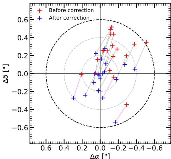
**Fig. 5.** Positional offset ( $RA_{HST} - RA_{ALMA}$ ,  $DEC_{HST} - DEC_{ALMA}$ ) between HST and ALMA before (red crosses) and after (blue crosses) the correction of both a global systematic offset and a local offset. The black dashed circle corresponds to the cross-matching limit radius of  $0''.6$ . The grey dashed circles show a positional offset of  $0''.2$  and  $0''.4$  respectively. The magenta lines indicate the HST galaxies previously falsely associated with ALMA detections.
