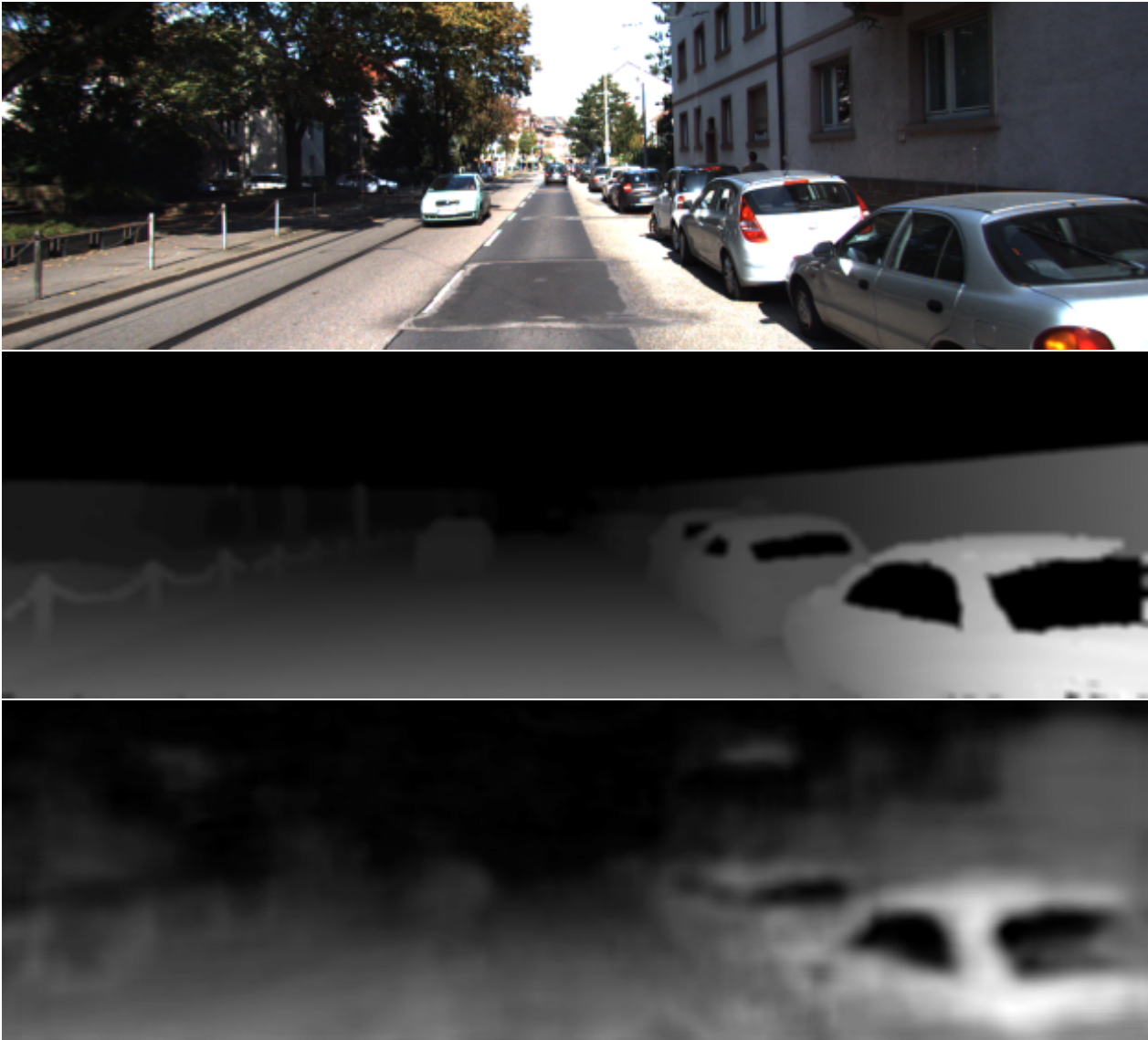
Figure 18. Stereovision test. Top: right image; middle: ground truth depth map for right image; down: predicted depth map.
