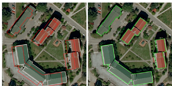
Figure 1. Multimodal matching. We align aerial images with cadastral images. Left: original misregistered images, right: after our realignment.
