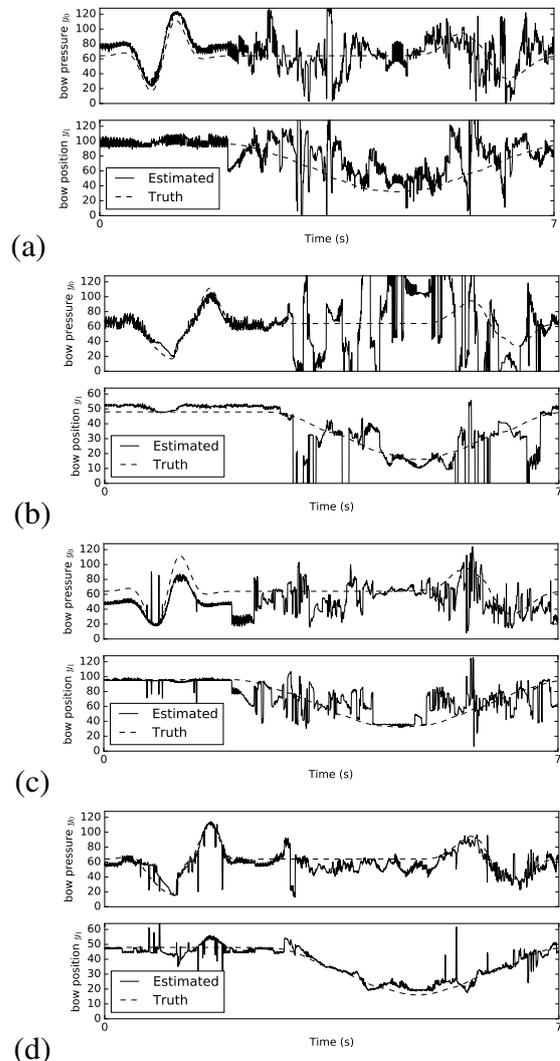
**Figure 3: Parameter estimation performance of the  $D1_Z2Y$  network for (a) *bowed1* full dataset, RMS error=23.23; (b) *bowed1* half dataset, RMS error=33.45; (c) *bowed2* full dataset, RMS error=19.54; (d) *bowed2* half dataset, RMS error=8.61.**
