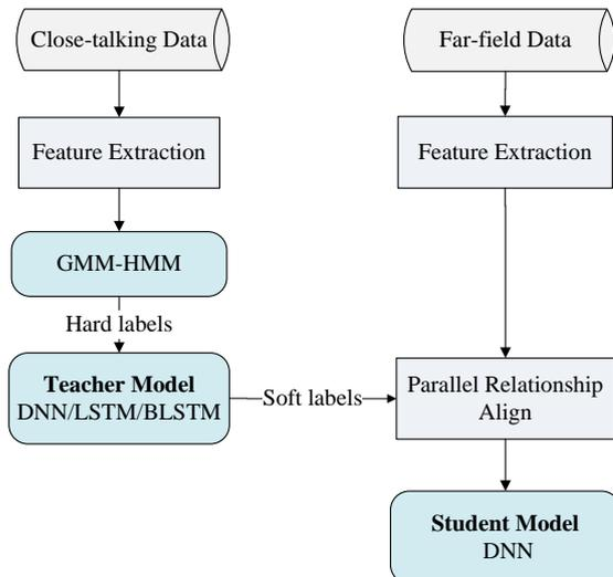
Figure 1: Framework of knowledge distillation for far-field speech recognition.
