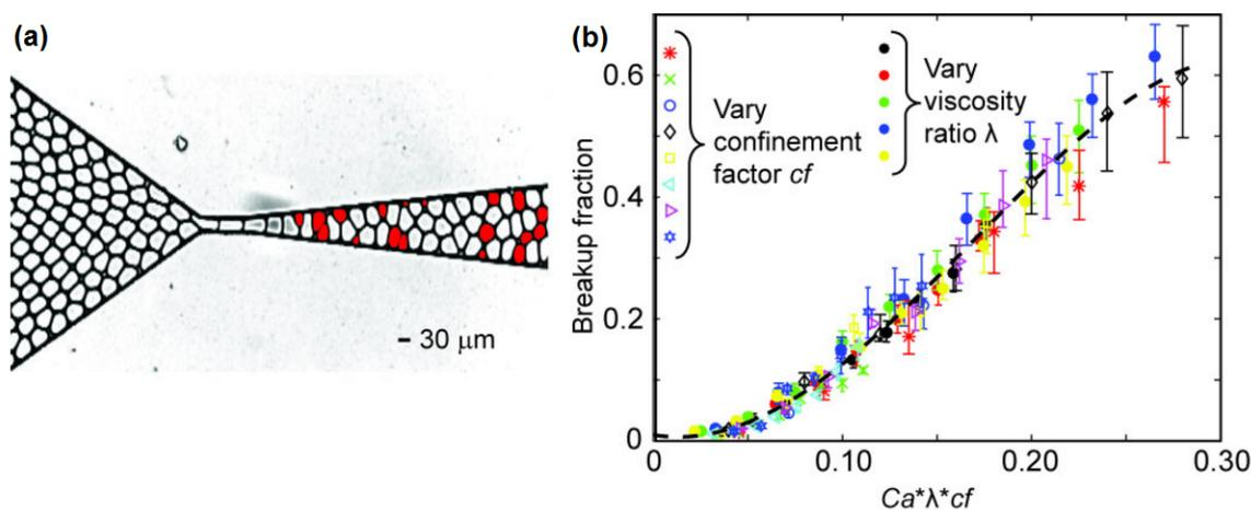
Figure 1. (a) Microscopy image of concentrated emulsion flowing in a tapered microchannel. Drops that underwent breakup after the constriction are highlighted in red. (b) Breakup fraction as a function of the product of capillary number ( $Ca$ ), viscosity ratio ( $l$ ) and confinement factor ( $cf$ ).
