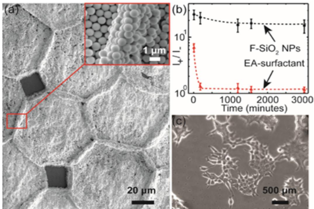
Figure 2. (a) SEM image of F-SiO<sub>2</sub> NPs stabilized droplets after evaporation of fluids. (b) Plots showing the time evolution of resorufin's fluorescence intensity ratio between positive droplets (contains 220 μM resorufin at t=0) and negative droplets (without resorufin at t=0). (c) Optical image showing the spread and growth of anchorage-dependent mammalian cells (MCF-7) after 19 hours of cultivation at F-SiO<sub>2</sub> NPs stabilized water/HFE-7500 interface.
