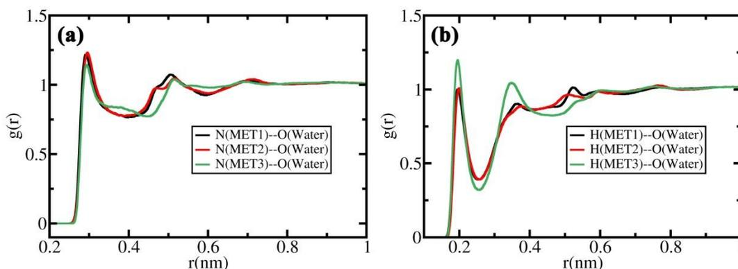
**Figure 9.** Radial distribution functions between certain atoms of metformin and oxygen atoms of water. (a) Pair correlation function between nitrogen atoms of metformin and oxygen of water. This shows two peaks  $\sim 3$ Å and  $5$ Å. (b) pair correlation function between acidic hydrogen atoms of metformin and oxygen of water. This shows two peaks  $\sim 2$ Å and  $3.5$ Å.
