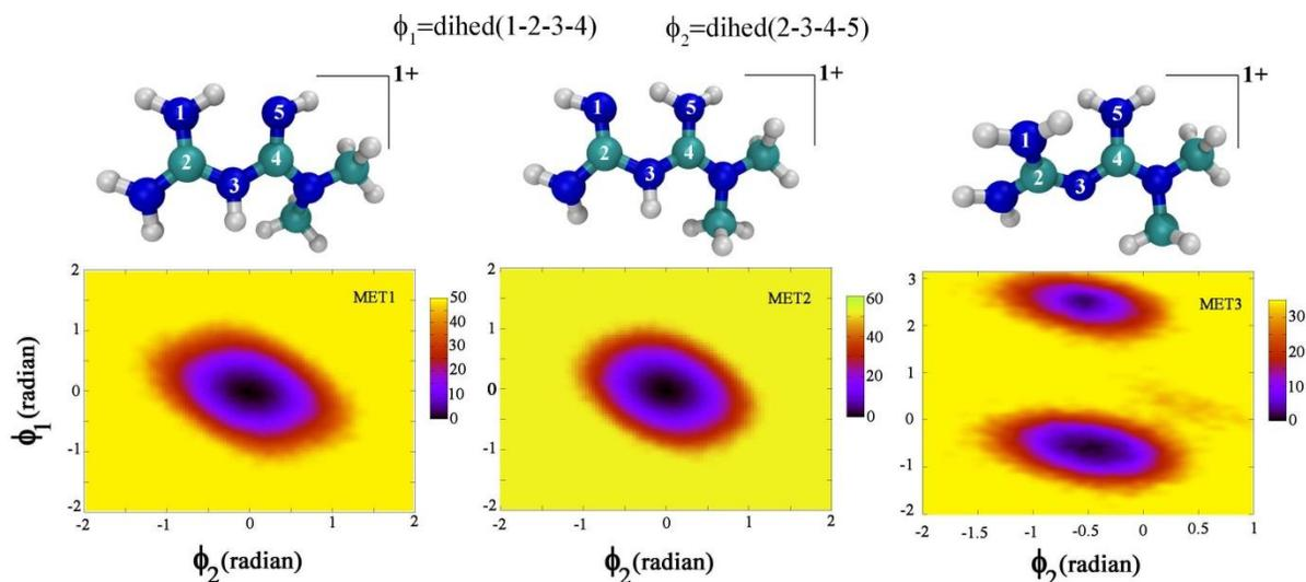
**Figure 6. Free energy (in kJ/mol unit) contours with respect to two dihedral angles ( $\phi_1$  and  $\phi_2$ ) of the three different mono-protonated forms of metformin hydrochloride. Because of the deep minima in free energy all three of them preserve the planar/non-planar conformation to a great extent under our force field description. In the timescale of performed MD simulations they are observed to evolve only in the deepest minima.**
