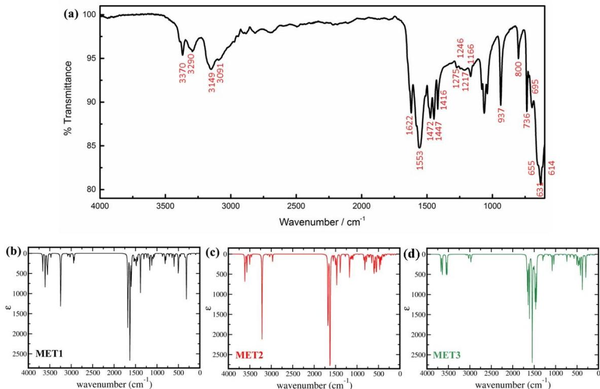
**Figure 4. Characterization of protonation states of metformin with the help of Infrared spectrum (a) experimentally and (b)-(d) with the help of quantum calculations on three different protonation states in implicit water solvent. It is clear that the tautomeric form resembles more with the experimental spectra. This again proves the dominance of the tautomeric form in the experimental sample.**
