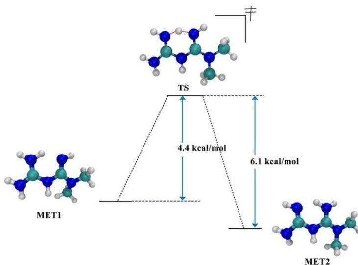
**Figure 7. Schematic representation of proton transfer reaction from one to another planar mono protonated form. The barrier crossing energy is low ( $\sim 4-6$  kcal/mol) which allows a possible co-existence of these two species in the solution.**
