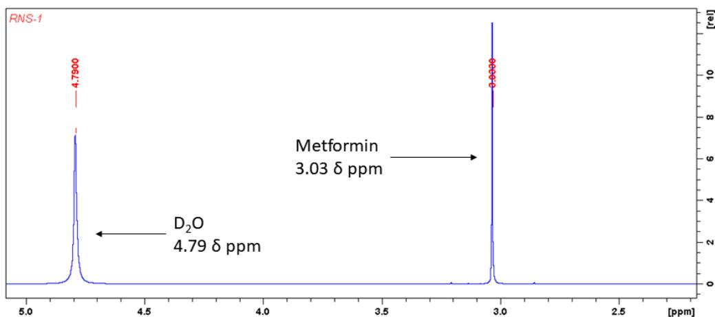
**Supporting Figure S1:** <sup>1</sup>H NMR spectrum of metformin crystals dissolved in D<sub>2</sub>O, showing the characteristic methyl protons at 3.03 δ ppm. The solvent peak is seen at 4.79 δ ppm.
