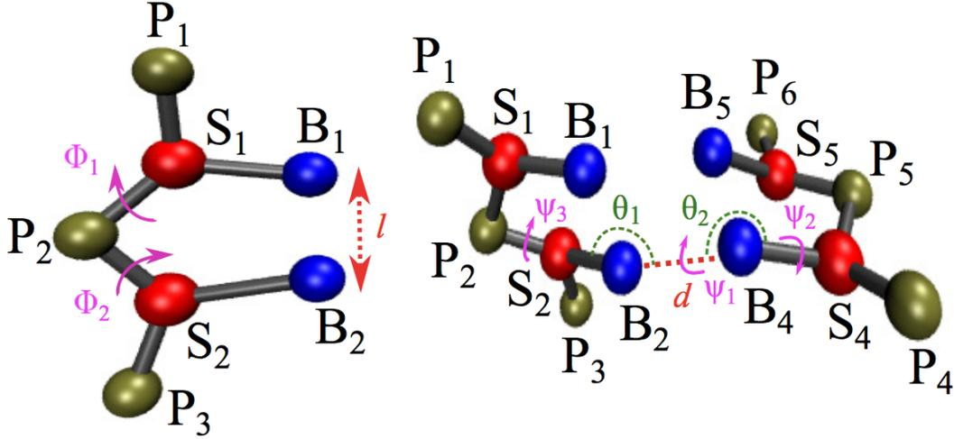
Figure 3: Left: Schematic of a coarse-grained dimer based on the TIS model, with  $l$ ,  $\phi_1$ , and  $\phi_2$  labeled. Right: Illustration of the structural parameters in equation (13). The hydrogen-bonding distance  $d$  is between sites  $B_2$  and  $B_4$ ;  $\theta_1$  ( $S_2, B_2, B_4$ ), and  $\theta_2$  ( $S_4, B_4, B_2$ ) are the angles;  $\psi_1$  ( $S_2, B_2, B_4, S_4$ ),  $\psi_2$  ( $P_4, S_4, B_4, B_2$ ), and  $\psi_3$  ( $P_2, S_2, B_2, B_4$ ) are the dihedral angles.
