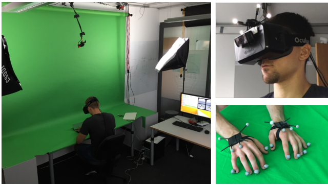
Figure 3: Left: Setup with green keying, tracking system and external lighting. Top right: HMD with external camera and tracking fiducial. Bottom right: fiducials used for tracking the hands in the IKHAND condition.
