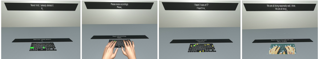
Figure 1: Views on the conditions studied in the experiment on effects of hand representations for typing in VR. From left to right: NoHAND, IKHAND, FINGERTIP and VIDEOHAND.
