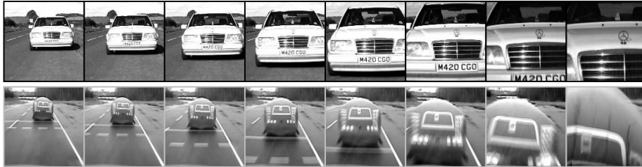
Figure 6: Video sequences showing object approaches Two video sequences which served as input I_t(x, y) to equation 14. The top row shows a couple of representative frames of a video where a car drives to a still observer. Except of some camera shake, there is no background motion present in this video. The car does actually not collide with the observer. In the video frames shown in the bottom row , a car (representing the observer) drives against a static obstacle. This sequence implies background motion. Here the observer actually collides with the balloon car, which flies through the air after the impact.
