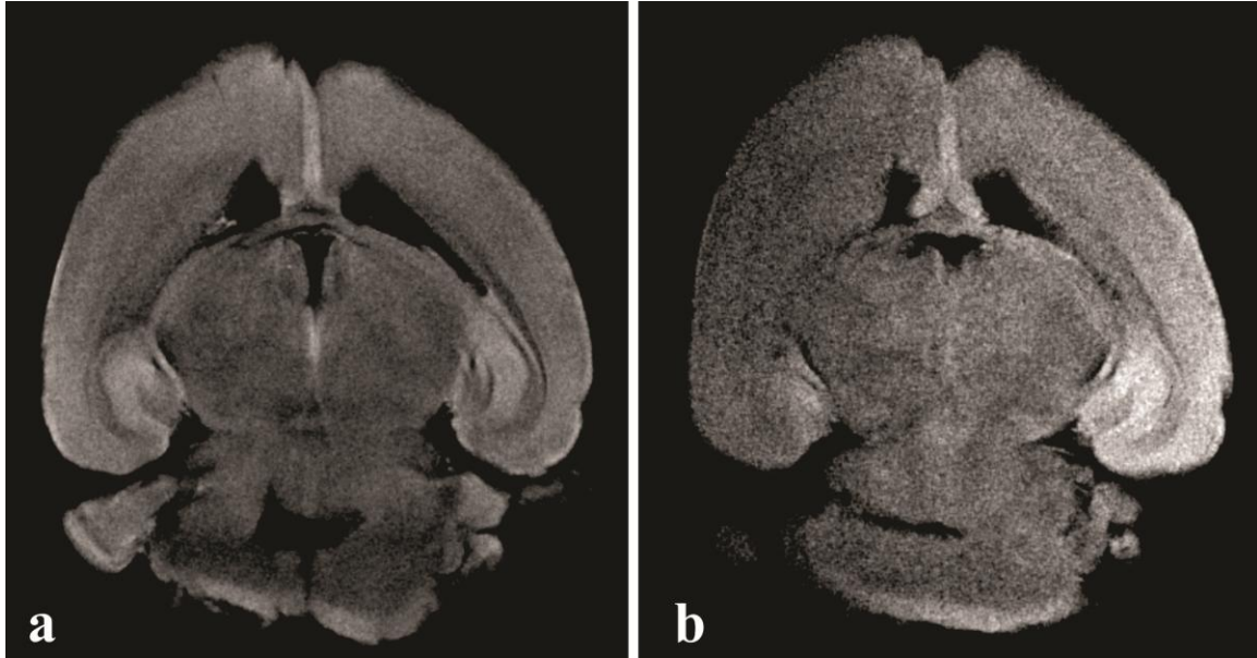
Fig. 3. Coronal slices from the mouse brain acquired with the LGR (a) and surface (b) coils using the following acquisition parameters: flip angle \alpha=82^\circ , TE = 3.4 ms, NEX = 1, FOV= 15 mm 2 , matrix size = 512×512 and TR=200 ms. Despite the use of identical acquisition parameters the LGR coil yielded 2× higher SNR .
