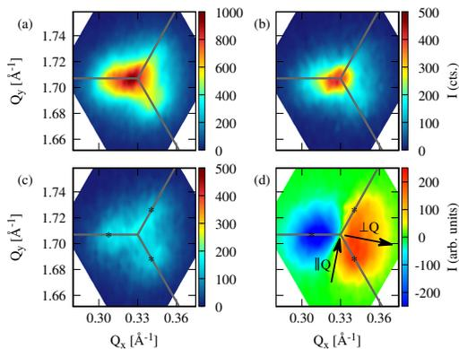
FIG. 5. The magnetic scattering at  $T = 4\text{K}$  near the  $(4/3, 1/3, 0)$  position with fine structure extending along the BZ boundaries: (a) total scattering, (b) contribution from spin components in  $ab$ -plane, (c) contribution from spin components in  $c$ -direction, (d) chiral signal reveals a purely cycloidal character exhibiting an antisymmetry perpendicular to  $\mathbf{Q}$ . Possible precursor of a long-periodic order are marked with \*.
