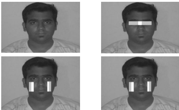
FIG. 5. FACE DETECTION USING VIOLA JONES ALGORITHM WITH RECTANGULAR HAAR FEATURE SELECTION
