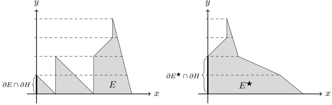
**Figure 2.** In general, the amount of perimeter on  $\partial H$  of a bounded open set  $E$  with polyhedral boundary is increased by the rearrangement defined in (3.3), so that  $P(E; \partial H) \leq P(E^\star; \partial H)$ . Precisely, the set  $\partial E^\star \cap \partial H$  coincides with the connected component of  $\{\varphi'_E = 0\}$  containing  $\partial E \cap \partial H$ .
