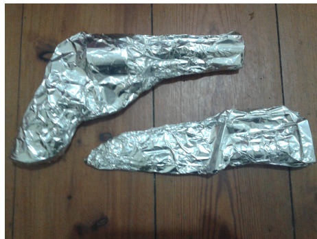
Figure 2: Plastic toy weapons covered with aluminium foil to increase the reflectivity is used for testing.
