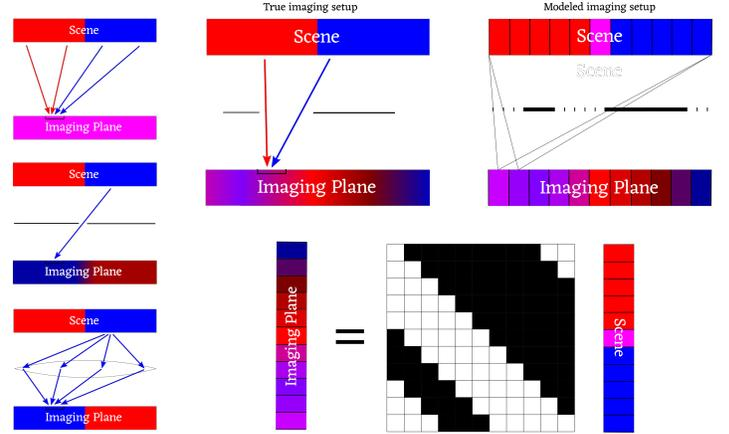
**Fig. 1:** Three imaging systems (left, top-to-bottom): no aperture, a pinhole and a lens. Arrows indicate paths light from the scene takes to a particular point on the imaging plane. On the right is an arbitrary mask, an illustration of its discretization and the corresponding transfer matrix.
