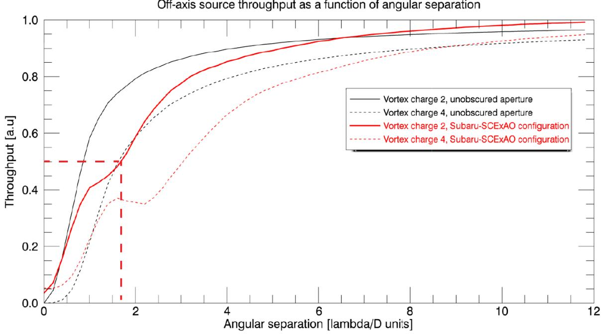
**Figure A1. Vortex coronagraph throughput in function of angular separation for the ideal unobstructed pupil charge-2 and charge-4 cases (black curves), and the real Subaru-SCEXAO configuration with a vortex charge-2 or charge-4 (red curves). The IWA (dashed red lines) of the current SCEXAO charge-2 vortex is  $1.7 \lambda/D$  (70 mas).**
