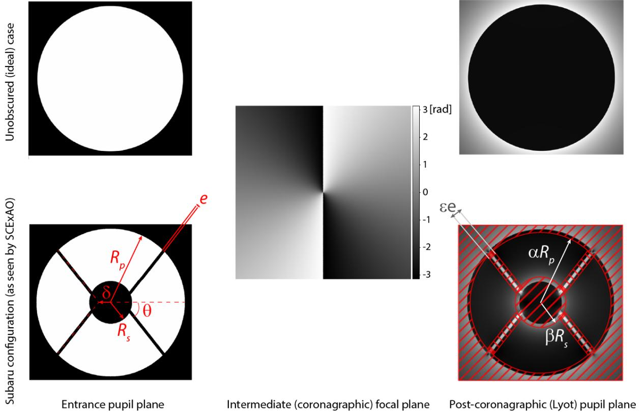
**Figure 1.** Principle of vector vortex coronagraphy for ideal (upper row) and Subaru-shaped (bottom row) telescope pupils, in the case of a topographic charge-2 phase mask. The Subaru pupil and SCEXAO Lyot mask parameters shown here are detailed in Section §2.3 and Table 2.
