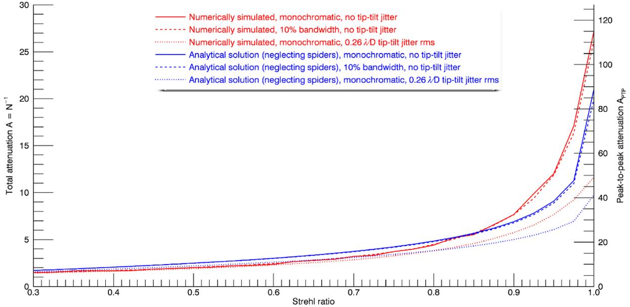
**Figure A2.** Numerically simulated (red) and analytical (Eq.12, blue) SCEAO vortex null depth performance predictions in function of Strehl ratio, in the diffraction-limited regime ( $SR > 0.3$ ). Various leakage contributors (see Annex) are added to illustrate their respective impact on null depth. The right-hand side  $A_{PTP}$  vertical axis assumes a coronagraphic PSF geometric scaling factor  $A_{PTP}/A \sim 4.2$ , but this quickly loses validity for  $SR < 1$ .
