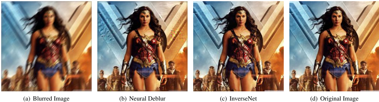
Figure 8. Motion deblurring for a 256 \times 256 image with model trained on 128 \times 128 images.
