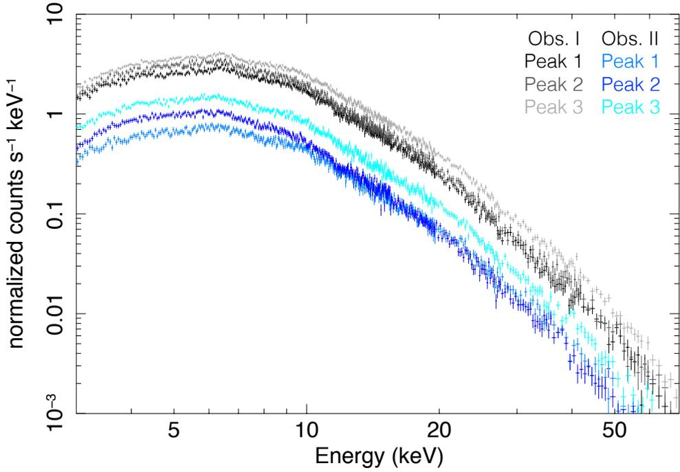
FIG. 6.— Spectra extracted from the three pulse-peak phase bins noted in Figure 4 for Observation I (greyscale) and Observation II (blues). Only the FPMA spectrum from each pulse peak is plotted, for clarity. While there are some differences in overall count rate, the slope of the power law is generally consistent across all three phase bins.
