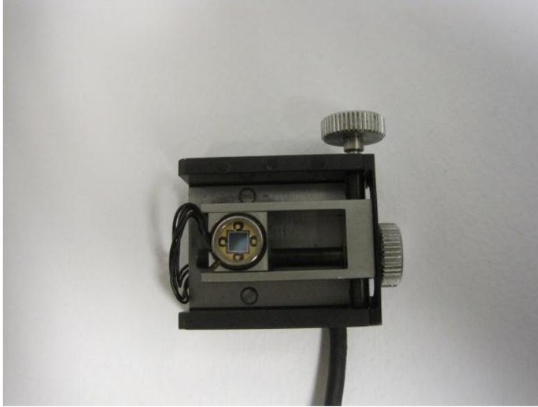
**Figure 2.1.3** Photodiode detector unit (bottom view) with photodiode chip “quadrant”
