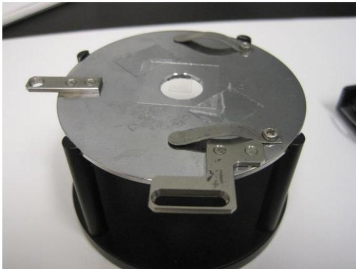
**Figure 2.1.2** Standard sample mounting stage (plate)
