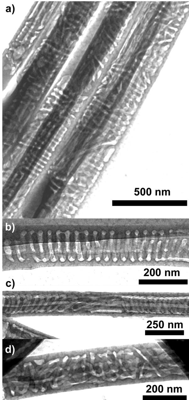
Figure 3: TEM images of released PS-*b*-PLLA nanorods ( $D/L_0 \approx 4.8$ ) after isothermal crystallization at  $T_C = 140^\circ\text{C}$ . The PLLA initially located at the positions of the voids was hydrolyzed. a) Overview. b)-d) Characteristic morphologies. b) Single hollow undistorted “low-pitch” helix with a pitch of  $\approx 40$  nm; c) distorted hollow helix surrounding a central hollow cylinder; d) disrupted concentric-lamellar morphology.
