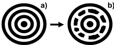
Figure 7: Sketch of cross-sectional views of PS-*b*-PLLA nanorods representing the structure evolution during annealing at 140°C (PLLA black). a) Initially, undisturbed concentric cylinder shells exist. b) During annealing, the cylinder shells formed by the second-outermost PS-*b*-PLLA layers are destroyed by an interplay of morphology ripening and PLLA crystallization.
