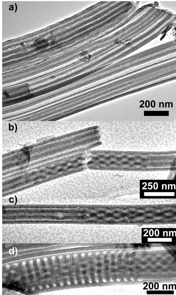
Figure 2: TEM images of released PS-*b*-PLLA nanorods after isothermal crystallization at  $T_C = 85^\circ\text{C}$ . The PLLA initially located at the positions of the voids was hydrolyzed. a) Overview. b-d) Examples of PS nanorods containing hollow helices in place of the PLLA domains; b), c)  $D/L_0 \approx 4.8$ ; d)  $D/L_0 \approx 7.3$ .
