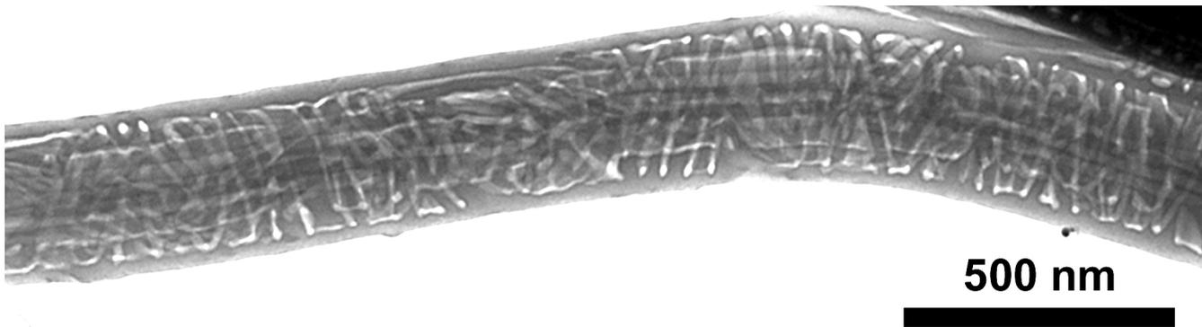
Figure 4: TEM image of a released PS-*b*-PLLA nanorod ( $D/L_0 \approx 8.4$ ) after isothermal crystallization at  $T_C = 140^\circ\text{C}$  in an AAO nanopore with a diameter of  $\approx 310$  nm. The PLLA initially located at the positions of the voids was hydrolyzed.
