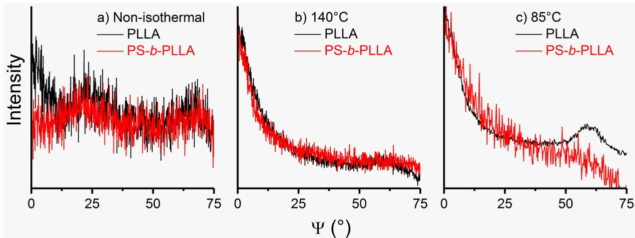
Figure 6: Normalized Schulz scans of arrays of PS-*b*-PLLA and PLLA nanorods located inside the aligned nanopores of self-ordered AAO ( $D = 180$  nm) for the (110)/(200) reflection of  $\alpha$ -PLLA a) after non-isothermal crystallization at  $-1$  K/min; b) after isothermal crystallization at  $T_C = 140^\circ\text{C}$  and c) after isothermal crystallization at  $T_C = 85^\circ\text{C}$ . The intensity of all Schulz scans in panels b) and c) is normalized.
