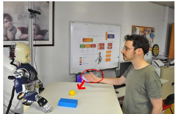
Figure 1: *Experimental setup, consisting of an iCub humanoid robot and a human user performing a manipulation gesture on a shared table with different objects on top. The depth sensor in the top-left corner is used to extract human hand coordinates for gesture recognition. Depending on the gesture and on the target object, the resulting effect will differ.*
