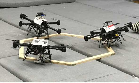
Figure 19. Experimental setup for the collaborative transportation of a bulky payload using three MAVs. The payload is an hexagon made of wood of 0.7 m of side length, weighting 2.46 kg. The distance between each MAV is approximately 1.2 m.
