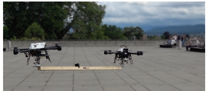
Figure 1. Experimental setup for outdoor collaborative transportation mission. The transported payload is a beam of wood, weighting 1.8 kg and 1.5 m long. The two robots are tightly coupled to the payload via a gripper with a spherical joint. During transportation, no communication is needed between the agents and all the algorithms are executed on-board.
