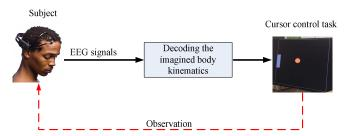
Fig. 1: A schematic of our EEG-based BCI platform for brain training and cursor control task
