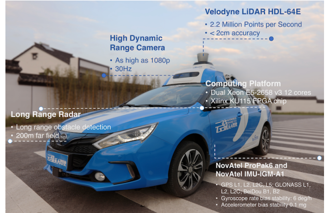
Fig. 1: Our autonomous vehicle is equipped with a Velodyne LiDAR HDL-64E. An integrated navigation system, NovAtel ProPak6 plus NovAtel IMU-IGM-A1, is installed for raw sensor data collection, such as GNSS pseudo range and carrier wave, IMU specific force and rotation rate. A computing platform equipped with Dual Xeon E5-2658 v3 12 cores, and a Xilinx KU115 FPGA chip with 55% utilization for LiDAR localization.
