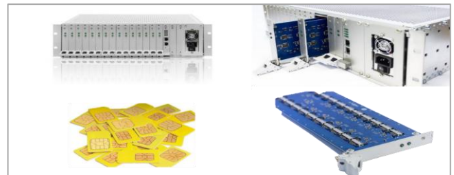
Fig. 4. A SIMbox and its components
