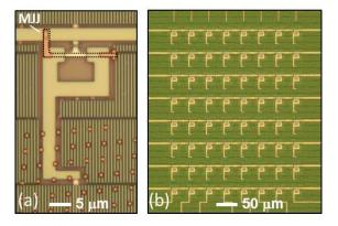
Fig. 4. (a) Optical micrograph of the unit cell and (b) an 8x8 array, prior to deposition of the final metal layer. The position of inductor  $L_3$ , which closes the storage loop in the top layer, is indicated with a dashed line in (a).
