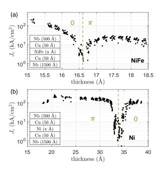
Fig. 2. Critical current density  $J_c$  of (a) Nb/Cu/NiFe/Cu/Nb and (b) Nb/Cu/Ni/Cu/Nb Josephson junctions vs magnetic barrier thickness. All data in each of the panels were measured on a single wafer, and the thickness gradient was produced by depositing the respective ferromagnetic metal at a 30 degree angle to the wafer normal. Regions of equilibrium 0- or  $\pi$ -phase are labeled according to Refs. [26] and [27].
