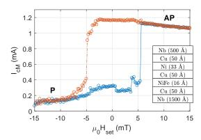
Fig. 3. Critical current of a 1  $\mu$ m $\times$ 2  $\mu$ m elliptical junction containing the layer stack shown in the inset. Measurements were performed at zero-field following the application of a set field shown on the x-axis. Blue (red) data points represent an increasing (decreasing)  $H_{set}$  sweep. The data trace the minor magnetization loop of the junction NiFe free layer.
