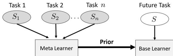
Figure 1. The meta-learner uses the data sets of the observed tasks  $S_1, \dots, S_n$  to infer ‘prior knowledge’ which in turn can facilitate learning in future tasks from the task-environment (which are unobserved by the meta-learner).
