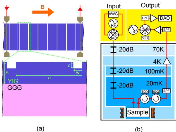
FIG. 1. (a) Simplified illustration of the magnonic crystal used in our experiments (not to scale). Here,  $S = 5.19 \mu\text{m}$ ,  $a = 300 \mu\text{m}$ ,  $w = 40 \mu\text{m}$ , and  $d = 0.5 \mu\text{m}$ . (b) Schematic of the measurement setup.
