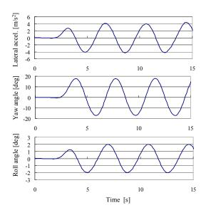
Fig. 3 Resultant vehicle motion in the simulations
