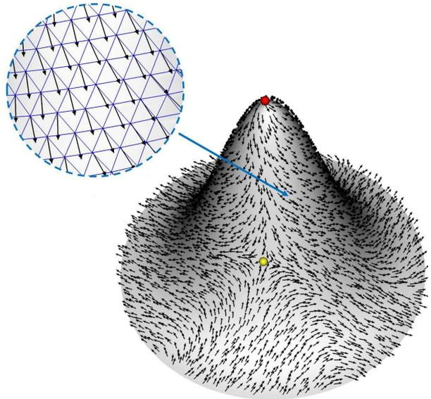
FIG. 1. Low temperature configuration ( $k_B T = 0.1J$ ) of the modified XY model obtained by Monte Carlo simulations on a Gaussian bump surface. In this relaxed configuration a positive vortex (red circle) locates on the top of the bump, and a negative vortex (yellow circle) down the surface. The inset shows a detail of the curved grid used in the simulations and the tangent vector field on this grid.
