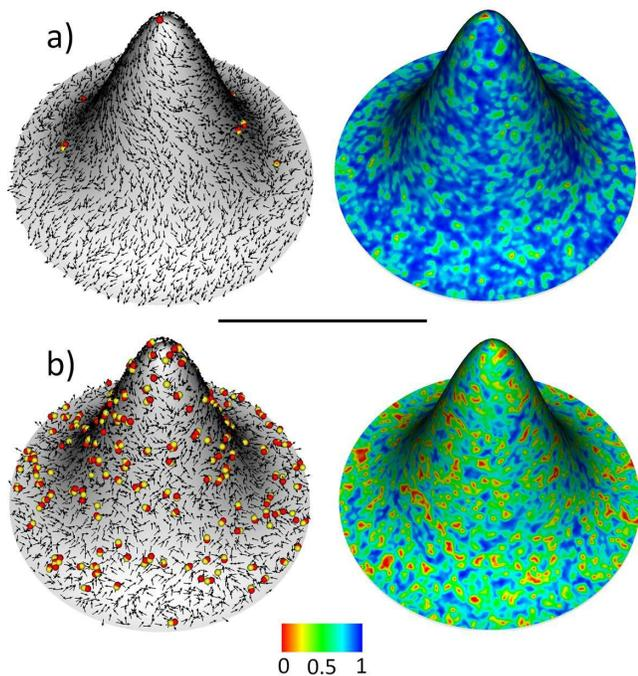
FIG. 2. Typical vector field configurations obtained by Monte Carlo simulations on a substrate of  $\alpha = 3$ , for low  $k_B T = 1.0J$  (a), and high  $k_B T = 1.75J$  (b) temperatures. The left panels show the vector field and the vortices, and the right panels show the corresponding short-range order maps and the color code used.
